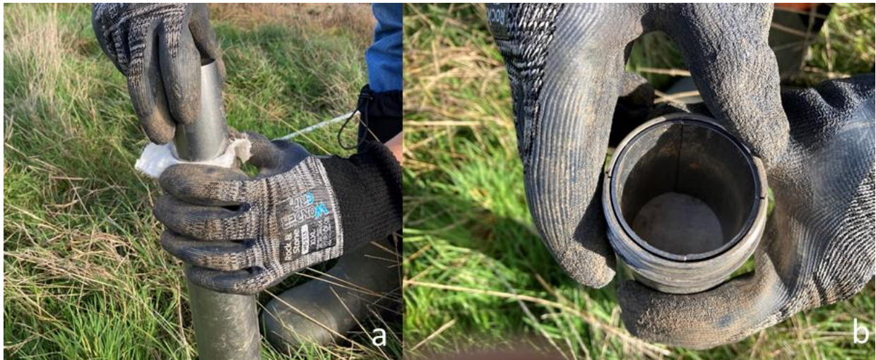
Figure 28: a) Inserting split liner into the corer before taking sample Z (spacer liner has already been placed inside the corer) b) Liner to take sample Z inside the corer with fabric mesh between the sample liner and the spacer.
