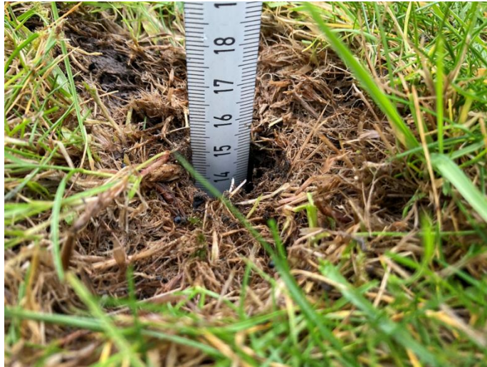
Figure 39: Measuring depth of hole to check if sample has been fully extracted for rA; if full extraction not possible record this in the app and mark on the bag (if conditions allow)
