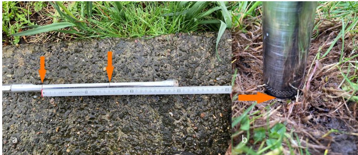
Figure 38: a) The small corer with 15 and 30 cm depth points marked, note the points are NOT where the stippled factory markings are (these are in inches). It is suggested that 15 and 30cm depths are marked on the corer using a marker pen and then more permanently with metal hacksaw for accurate sampling. b) Corer inserted to 15cm depth mark before extracting sample rA
