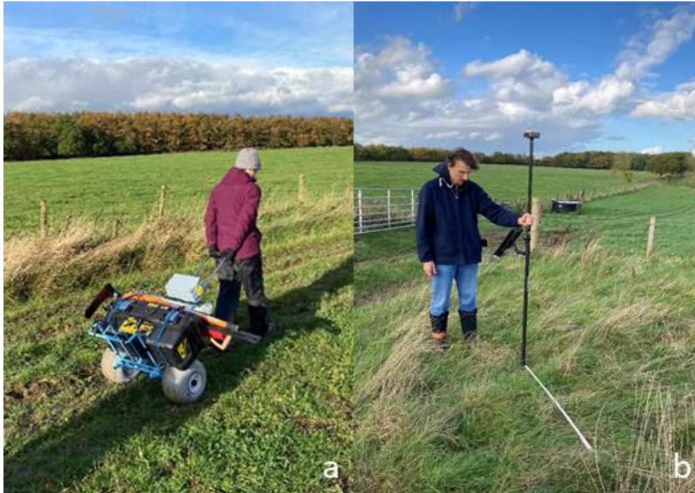
Figure 7: a) Transport of tools on a lowland site using a beach trolley b) locating the SW corner of sampling point using the GNSS receiver and an iPad mounted on a survey pole.
