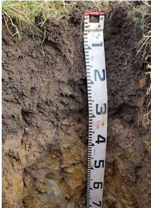
Figure 16: A soil profile where topsoil depth is 30cm (scale in decimetres).
