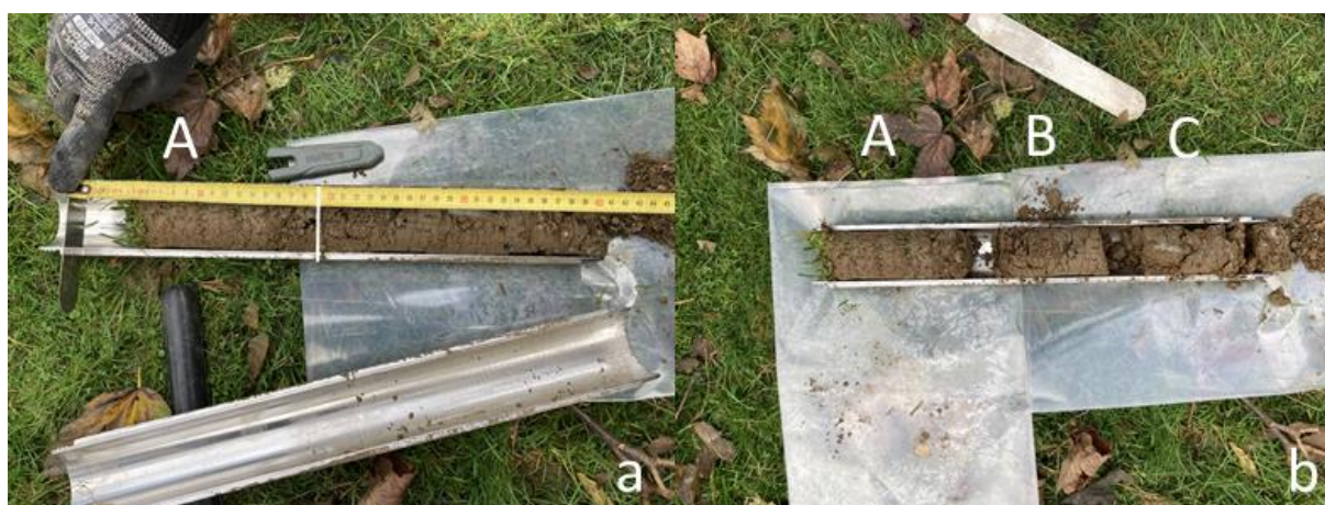
Figure 33: a) Example of compression in sample A; b) segmented sample.
