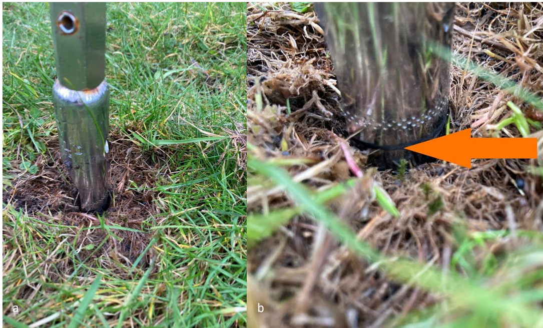
Figure 41: a) Sample inserted to 30cm to take sample rB in the same hole sample rA was taken from. b) Close-up of correct depth for sample rB – note black mark below the stippled factory mark.
