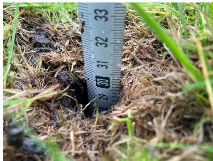
Figure 42: Measuring depth of hole to check if sample has been fully extracted for rB; if full extraction not possible record this in the app and mark on the bag (if conditions allow)
