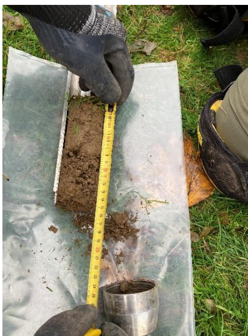
Figure 36: Sample M, photo illustrating minor compression of the sample.
