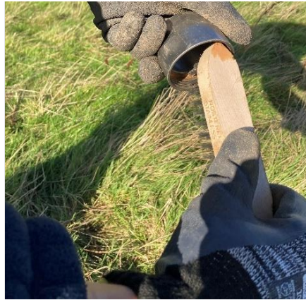
Figure 19: Cleaning the threads inside the core tip with a wire brush to remove excess soil
