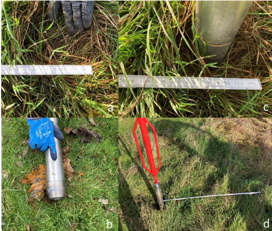
Figure 29: Examples of placement of corer for sample Z a) low and soft vegetation parted by hand b) 8 cm mark on corer – sampling depth c) placement of corer on surface d) soil corer in position before sampling.
