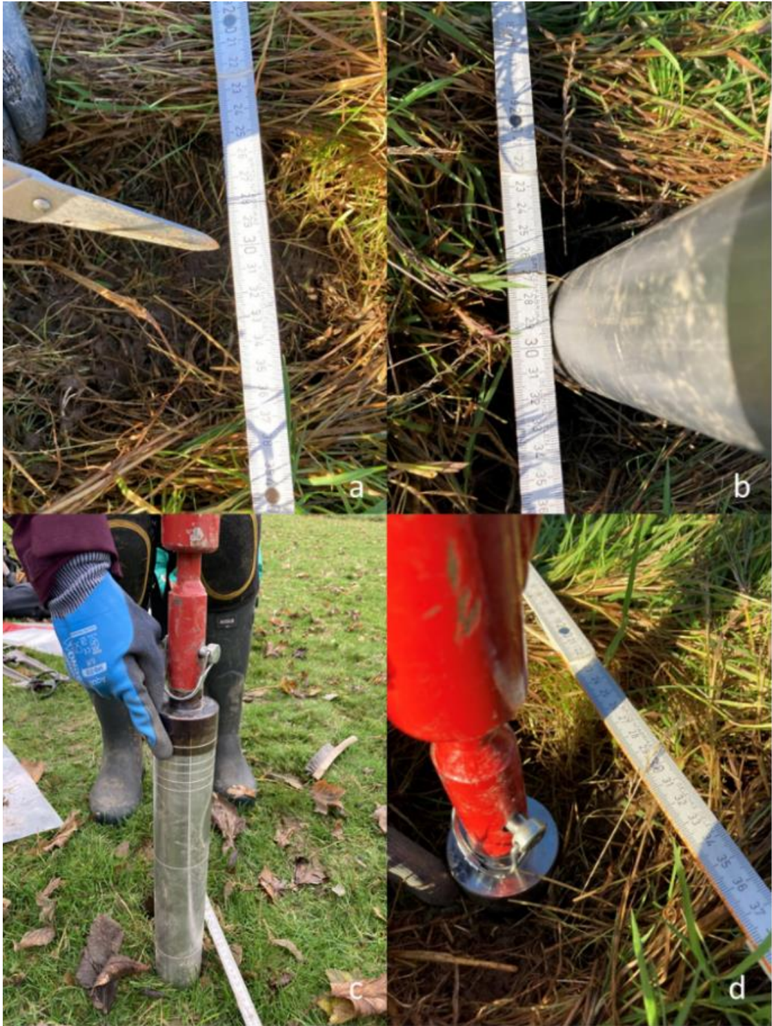
Figure 32: a) Vegetation removed from sample area b) Corer placed at 30 cm on the NE axis on the soil surface c) 43 cm marker on the corer d) Corer inserted to 43 cm depth.
