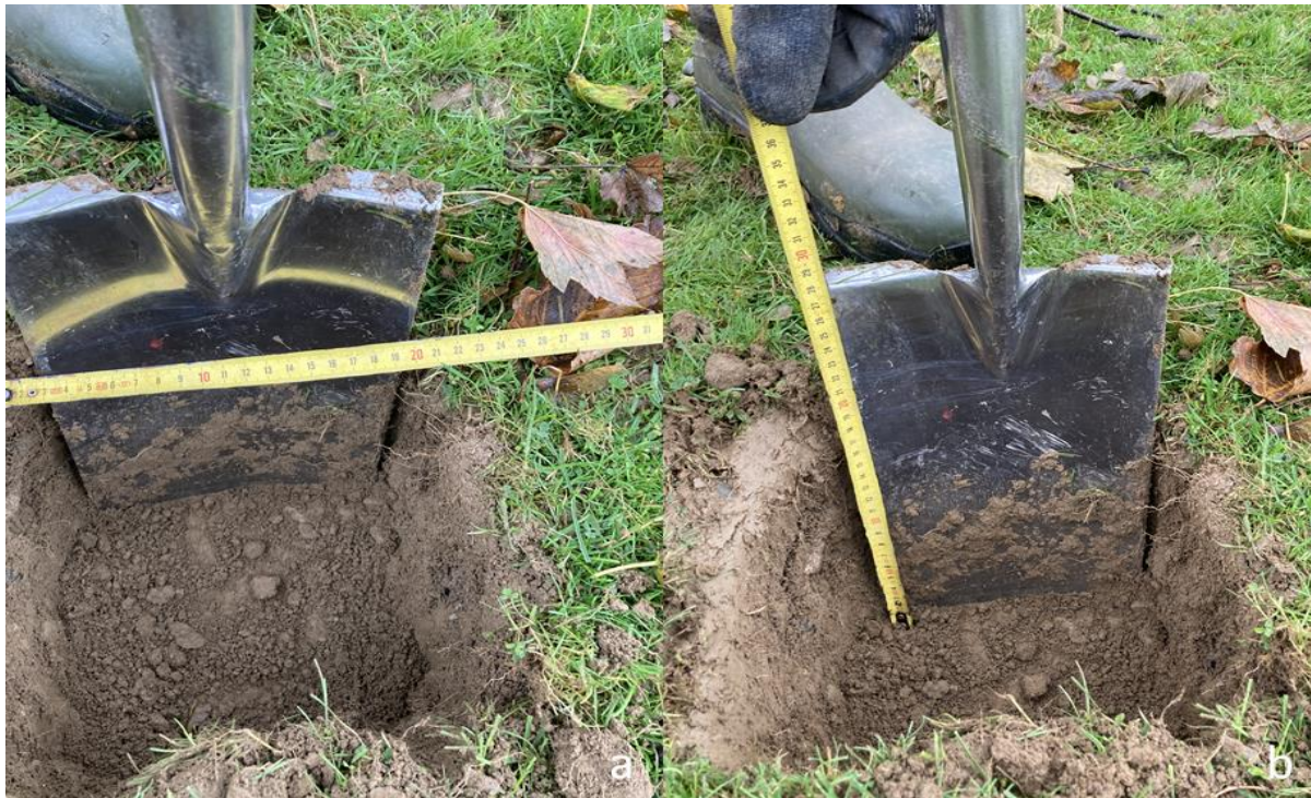
Figure 15: a) Width and length of square (20cm x 20cm) and b) depth of excavated block (20cm)
