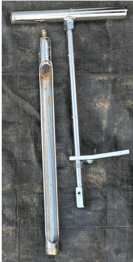
Figure 37: The small corer for mycorrhizal sampling has a T-handle, extension rod, foot jack and soil sampling tube.
