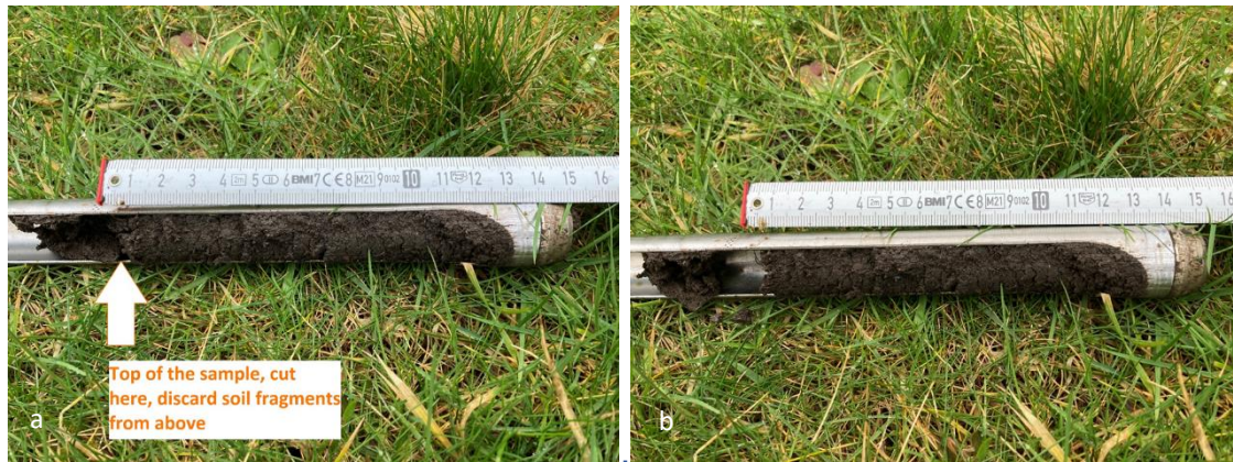
Figure 43: a) Sample rB after extraction, note loose soil originating from above the sample that needs to be discarded. b) Sample rB, soil fragments from above depth of 15cm separated, note slight sample compression.
