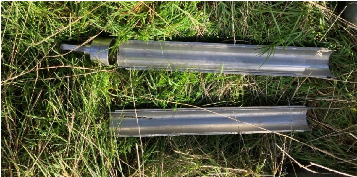
Figure 27: Spacer plastic tube in the corer before assembly (steel spacers provided in your toolset).
