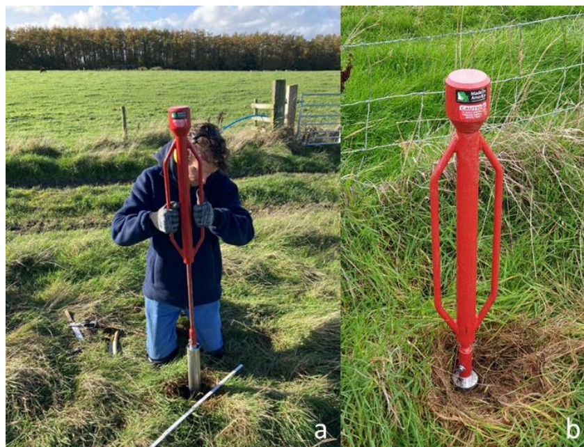
Figure 20: a) Soil sampler driving core into the soil using slide hammer (10kg hammer). Lighter version available for upland and remote sites where use of trolleys is not possible. b) corer inserted at full depth of 45cm (sample length) with hammer still attached.
