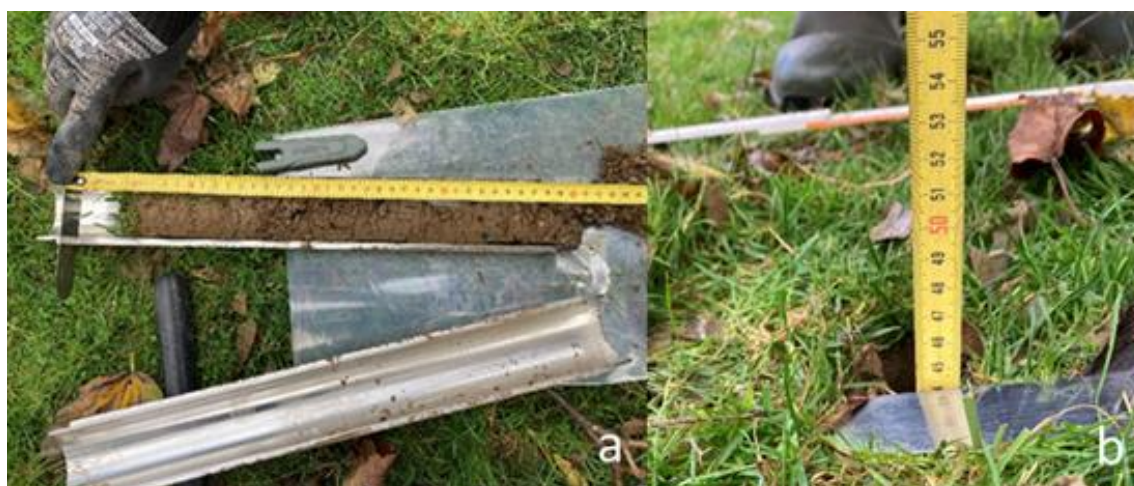
Figure 24: a) Illustration of sample compression b) Illustration of measurement of the sampling hole to check for sample recovery
