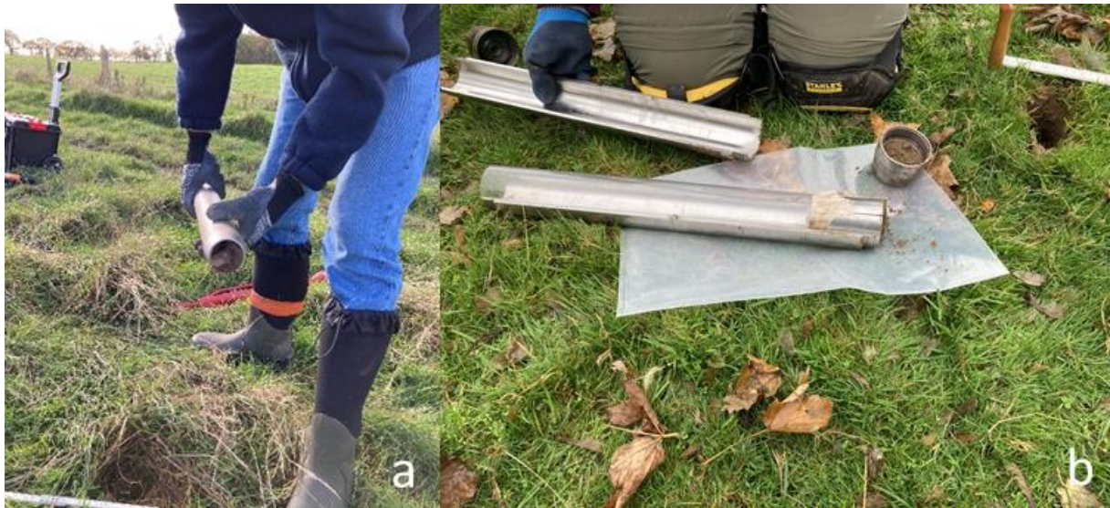
Figure 30: Sample Z after the sample has been taken a) check bottom of corer if soil has been pulled out b) sample slightly pushed out of corer
