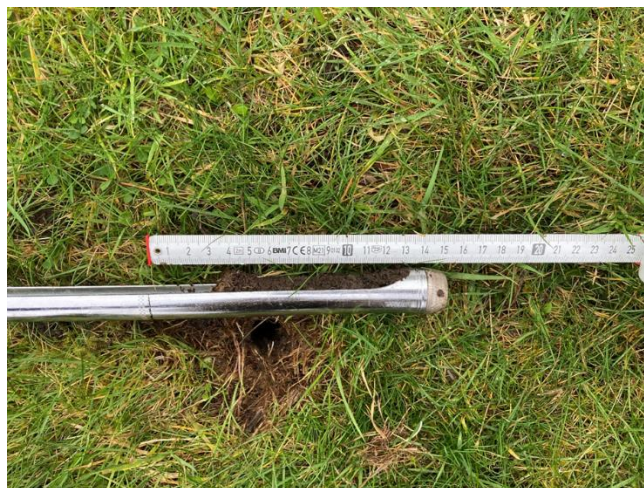
Figure 40: Sample rA after extraction, note compression.
