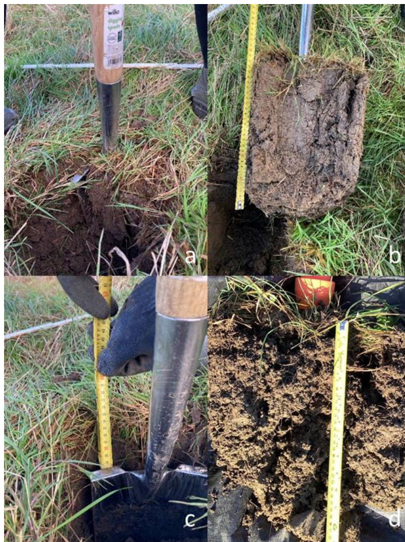
Figure 17: Examination of soil structure in a block excavated using a spade. a) visualisation how deep the spade should be inserted next to excavation hole of sample W b) excavated block c) showing depth of hole in relation to length of spade blade d) block loosened up to visualise soil structure before taking a photograph (detailed method in Appendix 4).
