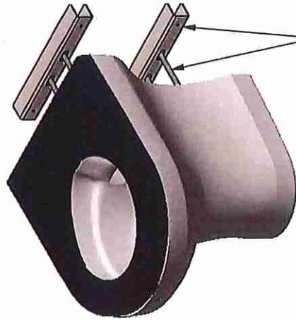
(A) WALL FIXINGS M10 X 225mm (4 OFF), & CLAMP BRACKETS (2 OFF).
