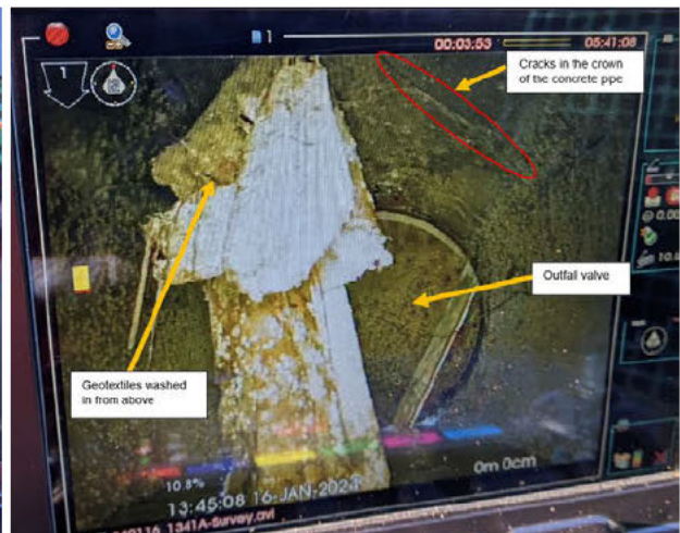
Figure 9- CCTV image (01/2024) taken from penstock chamber towards outfall.
