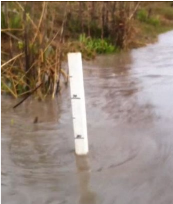
Figure 1: A graduated marker pole used to provide a measurable estimate of wave height.
