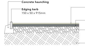
Surface course 25mm 6-10mm hardstone to match existing in bitumen binder
