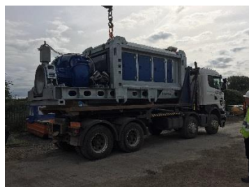
Lorry 4 - BBA pump on Hooklift Truck/Loader
