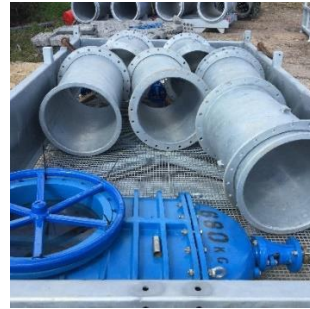
Stillage 4 –600mm pipe, valve, A/valve & vacuum breaker
