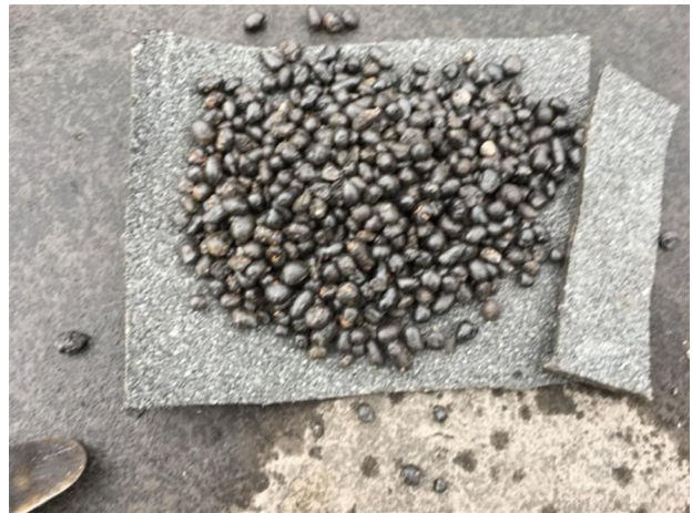
Close up image of lightweight screed
