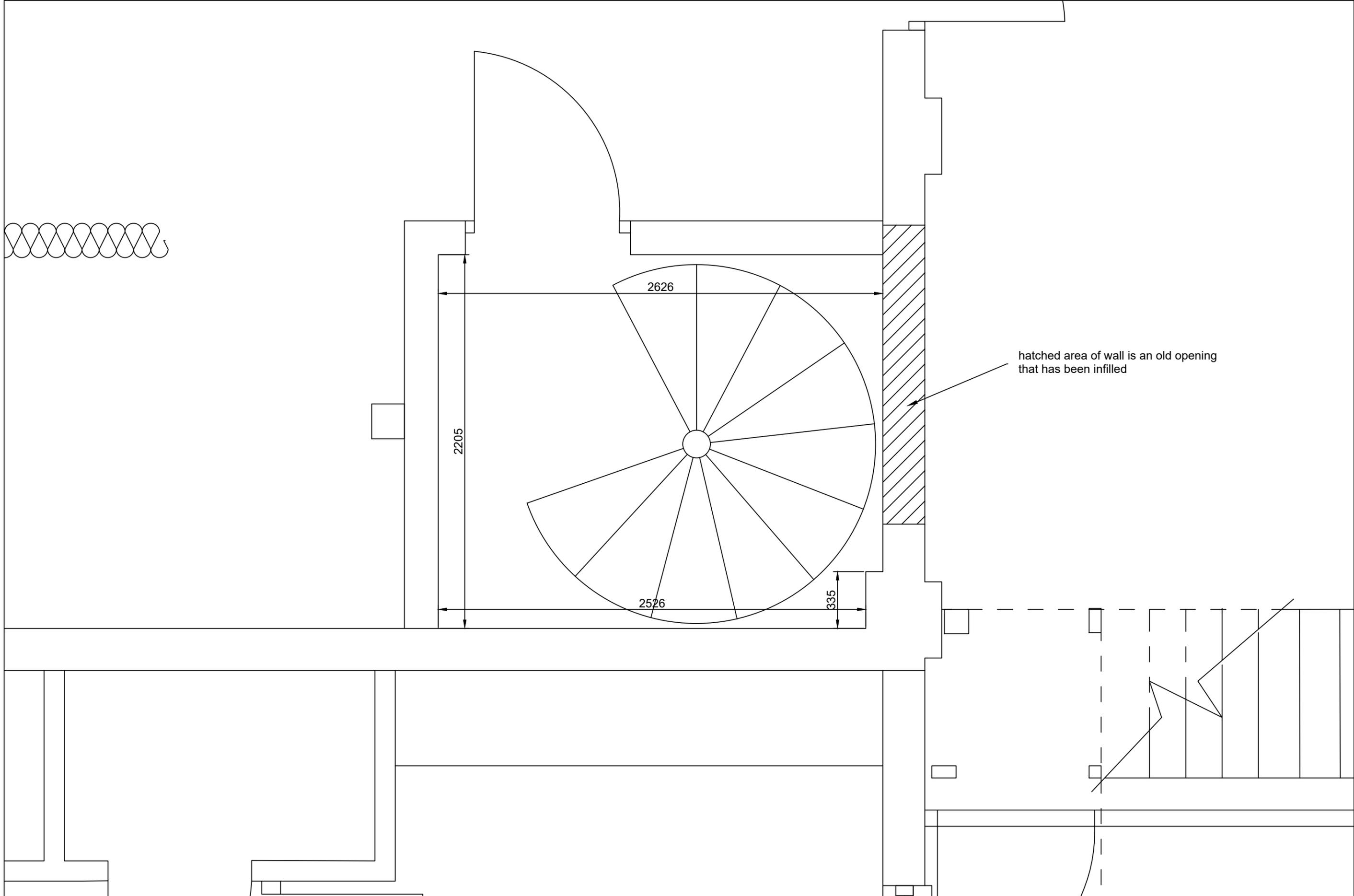
hatched area of wall is an old opening that has been infilled
