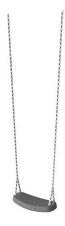
The KOMPAN swing seat is specially designed for children. It has a curved shape with a non skid surface of thermoplastic elastomers (TPE) which is moulded on an insert of polypropylene (PP) plastic. The combination of these two types of plastic gives a high value seat with a soft, user friendly surface. The seat is attached to the swing by use of Y-chains.
