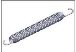
All 36 springs are made of stainless steel to ensure durability and excellent corrosion resistance. The steel wire is 3,2 mm thick and the last five windings are cone shaped to ensure long lifetime of the jumper.
