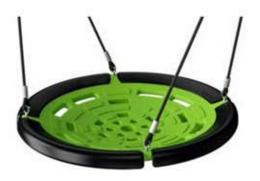
The shell seat is made of 100% recyclable polyethylene (PE) and rotomoulded in one piece. The seat is designed with large outer openings for handholds and middle holes for drainage of water and dirt. The four ropes are attached with hot dip galvanised steel brackets to ensure durability for many years.
