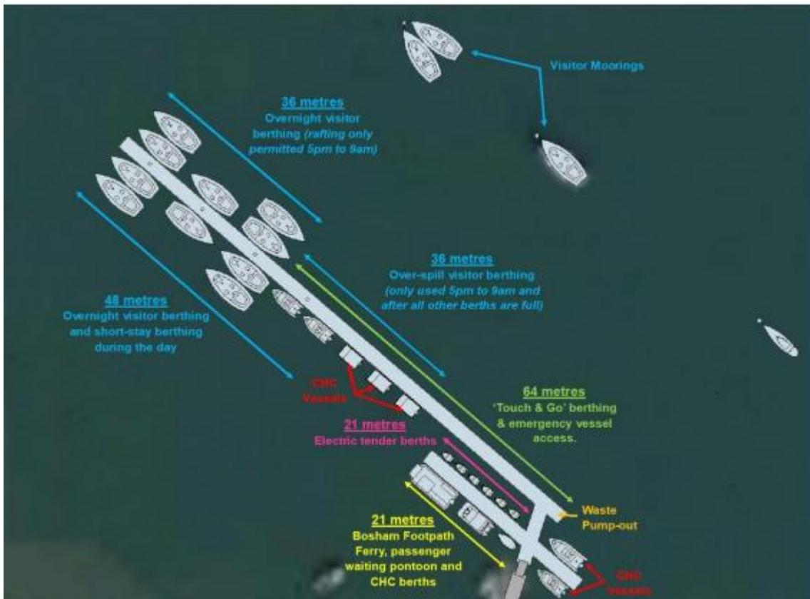
Figure one: Final overall design of the jetty.
