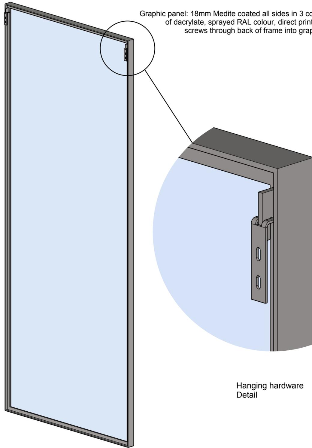
4mm steel frame, powdercoated RAL 7036
