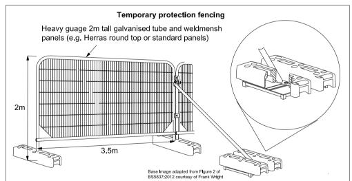
To prevent compaction within Root Protection Areas (RPAs) and mechanical damage to the above ground parts of retained trees during construction, appropriate protective measures must be installed prior to and for the duration of the development. This will be achieved by the creation of Construction Exclusion Zones (CEZs) protected by barriers as specified in Figure 3 of BS5837: 2012 (see above).
