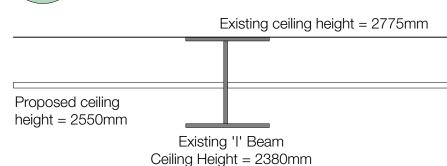
Proposed ceiling height 225mm lower than existing for any/all mechanical and electrical services. Allowance to be made for finishes/paint work to the remaining exposed 'I' beam.
