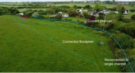
A pilot channel will be excavated, to pass water under the raised footpath route.
