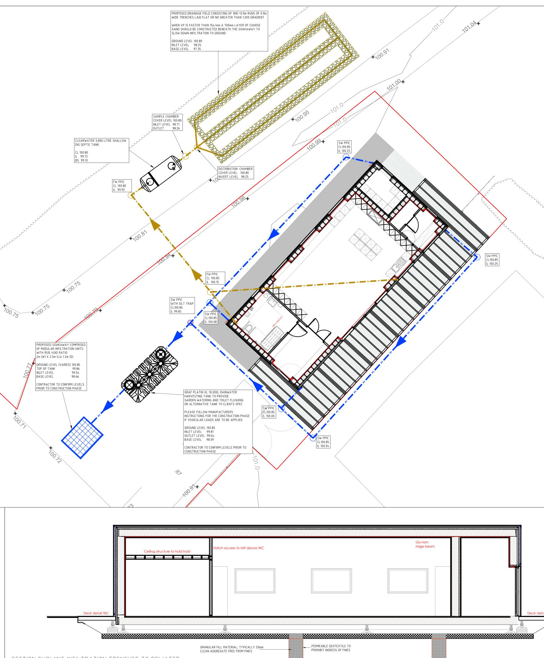
SECTION SHOWING INFILTRATION TRENCHES TO DEWA SUMP BELOW BUILDING
