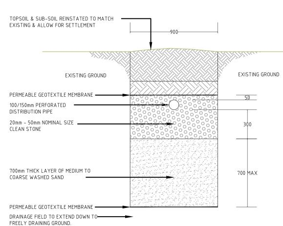
MODIFIED SECTION THROUGH DRAINAGE FIELD TRENCH1:20
