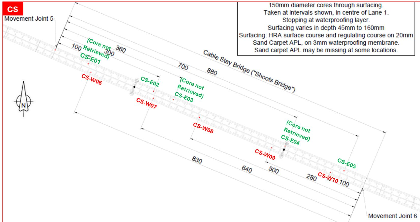
150mm diameter cores through surfacing.
