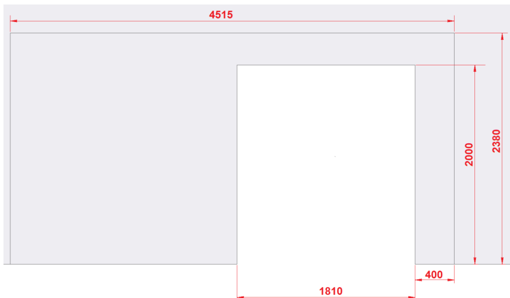
Figure 8 – Approximate geometry of existing wax tank
