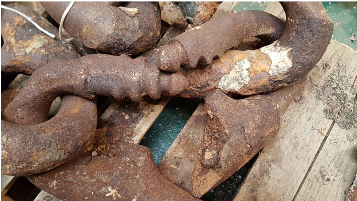
Figure 4 Example of Damaged Baldt cable (02)
