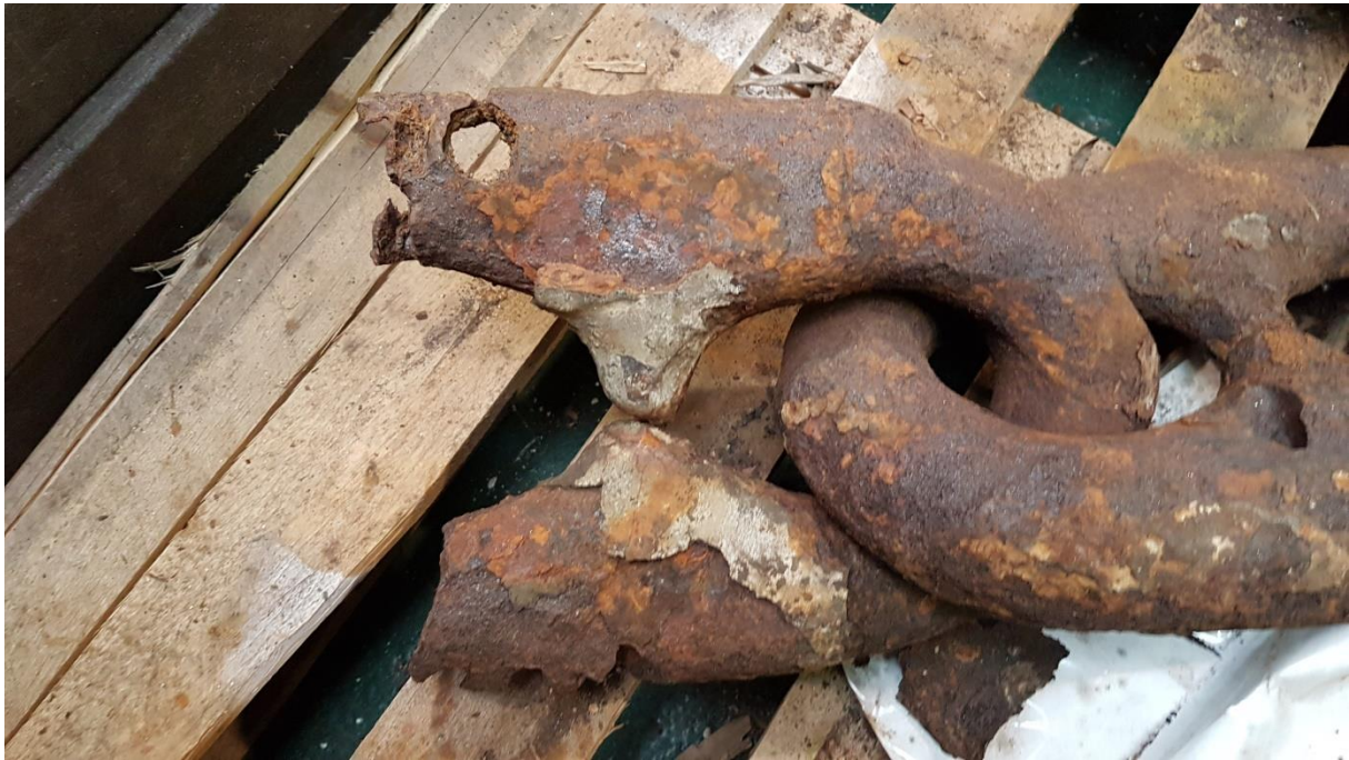
Figure 5 Example of Damaged Baldt cable (03)
