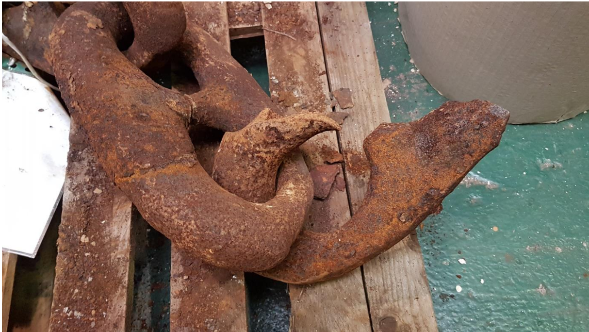
Figure 3 Example of Damaged Baldt cable (01)
