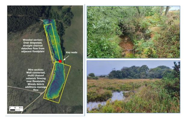
At the transition between the mire section and the wooded section there is a key point where water becomes concentrated into the incised, over deepened channel and consequently becomes disconnected from the natural floodplain. Water level changes at the transition point and falls by in the order of 1m as a cascade which coincides with tree roots/wood in the channel.
