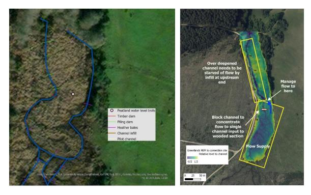
The central channel is deeply incised and significantly removed from the floodplain. A plausible explanation for this is that the steep drop in levels at the waterfall (key node) just downstream (see wooded incised section), is having a knock-on erosion effect, dragging the base level down towards the level of the deeply incised ditch below.
