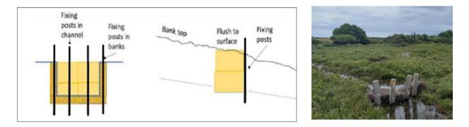
The intention of the blocks is to cause backing up of flow which then spills outside of the channel onto the adjacent valley floor, creating shallow flow over the surface.
