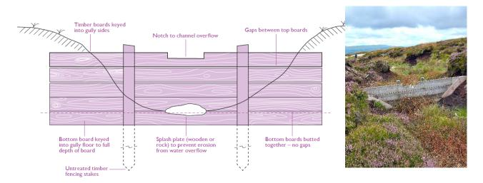
The timber board dams will be fixed in place by digging boards into the banks of the channel and using fence posts on the downstream side, in the banks and within the channel to secure them. These are not dams that we want water to flow over or around, but should act as blockades, which funnels the water past the existing routes on its way to the natural floodplain.
