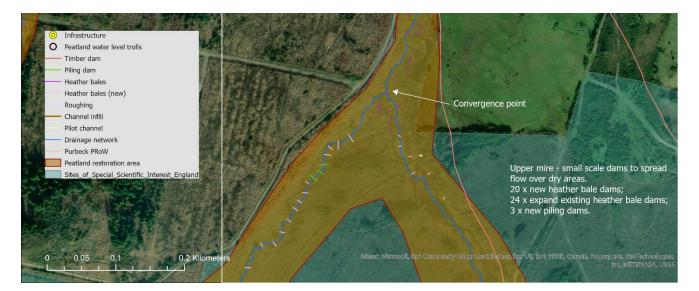
a) Maintain existing dams (24) – raising the height and expanding the width where required. Existing dams (built to date by volunteers) have been reviewed for extensions/maintenance. 24 dams have been constructed and require around 90 bales and 50 chestnut stakes to sufficiently expand them. Locations of these dams have been mapped for reference. The heather bales will be sourced and provided to the contractor. The contractor will provide the chestnut stakes.
