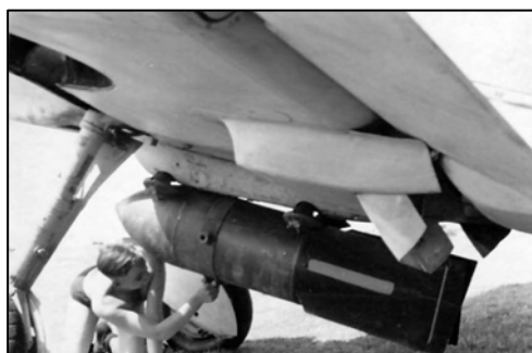
SC250 attached to undercarriage of Messerschmitt Bf109
