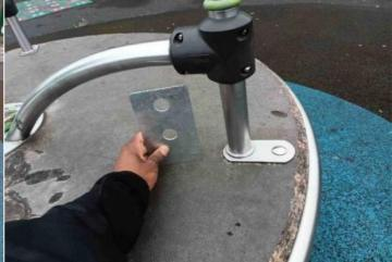
Finding: The item fails to meet the requirements of BS EN Action: Monitor - No remedial work recommended 1176 Part 1 4.2.7.2 for head and neck entrapment in the handgrip
