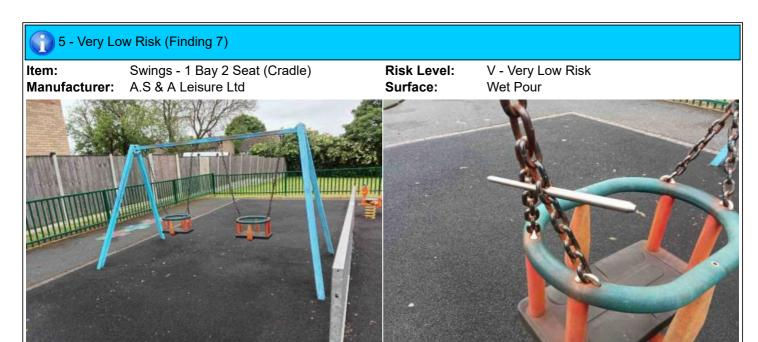
**Finding:** The chain openings are in excess of the 8.6mm as **Action:** Monitor - No remedial work recommended recommended by BS EN 1176
