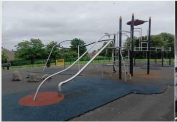
**Finding:** There is/are finger entrapment/s in the platform and the item fails to meet the requirements of BS EN 1176 Part 1 4.2.7.6 Entrapment of fingers
