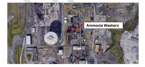
The use of the appropriate technology and consideration of remote machine/mechanical intensive means to demolish the ammonia washers, in order to reduce the impact of personnel working in close proximity to the ammonia washers, should be prioritised.
