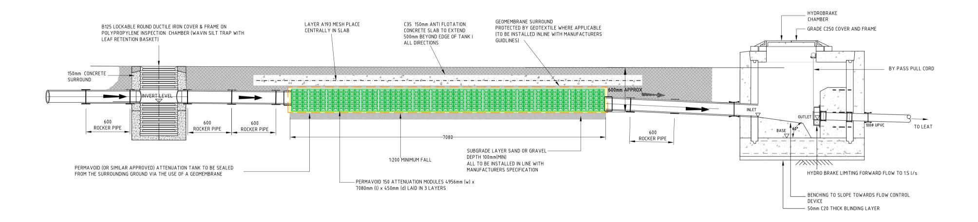
TYPICAL SECTION THROUGH SURFACE WATER ATTENUATION TANK AND HYDROBRAKE
