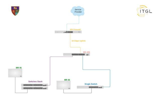
A single MS425 core switch will handle fibre and copper uplinks from the edge switches, up to 10 Gbps each.
