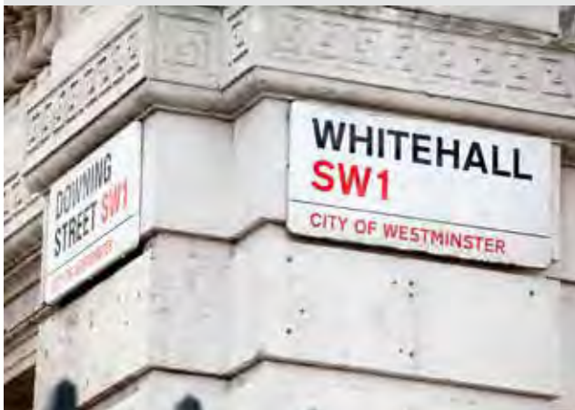
Figure 253: Street name plates should provide strong visual contrast between lettering and the background
