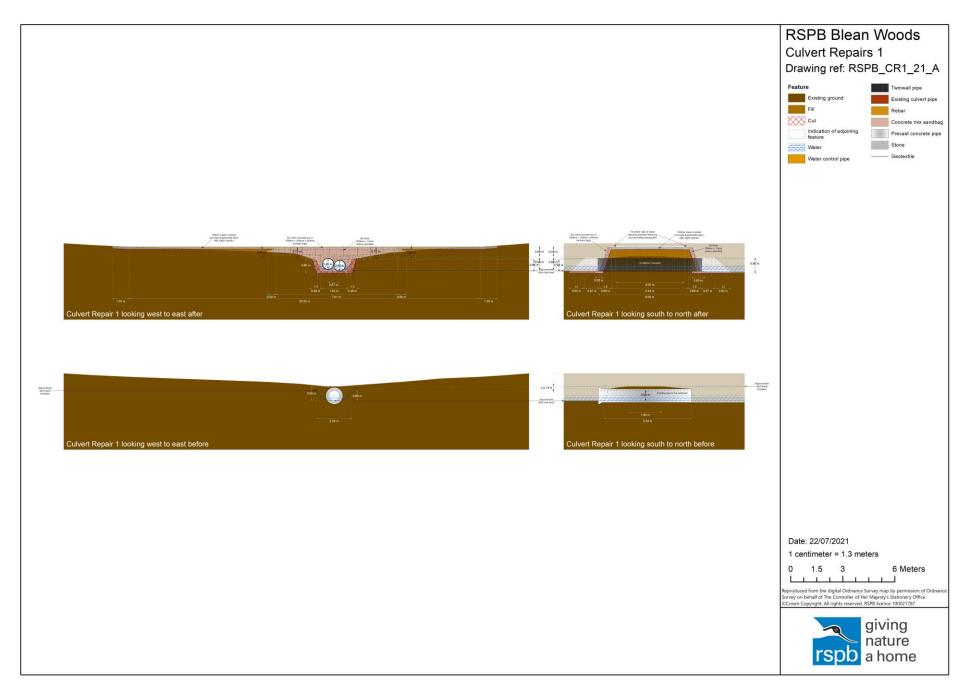
Figure 3 1a.2 Design drawing for culvert repair 1
