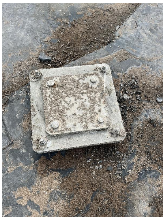
Figure 5: Mounting pole fixed plate with removable protective cover (left) and the Leica P40 Laser scanner on mounting pole (right)
