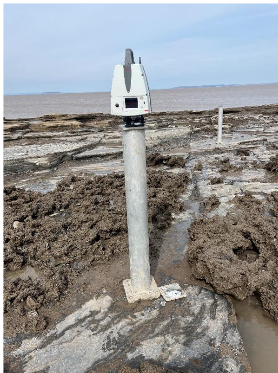
Figure 5: Mounting pole fixed plate with removable protective cover (left) and the Leica P40 Laser scanner on mounting pole (right)
