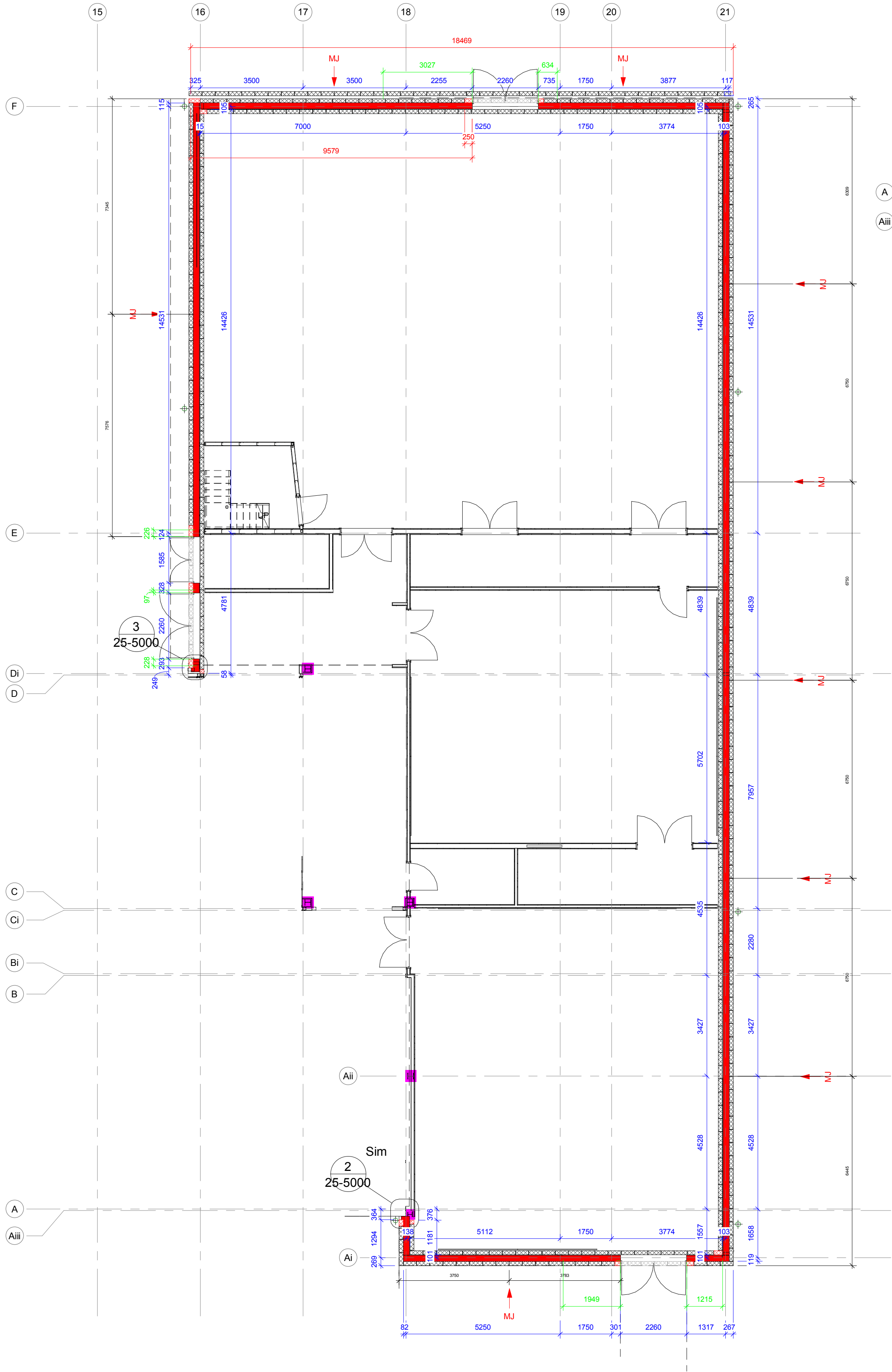
1 00 Ground Floor - Traditional Blockwork Setting Out 1 : 100
