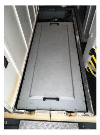
Modification 1 – Picture number 8. This picture is of CPV Alert before modification. Seen in picture grey (battery box). Needs moving forward approximately 12 cm allowing better access to the bilges.
