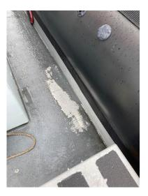
Defect 4 – Picture number 5, number 6 and number 7. Deck to superstructure sealant
