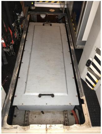
Modification 2 – Picture number 9. This picture is of the proposed modification that has been made on another CPV. This would be the outcome after modification providing equal space either side whilst not introducing any restriction.
