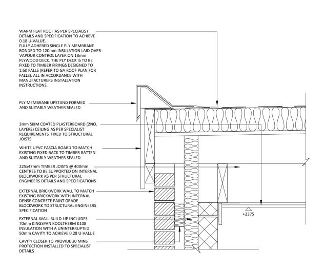
DETAIL 1 - FLAT ROOF AND EXTERNAL WALL JUNCTION DETAIL
