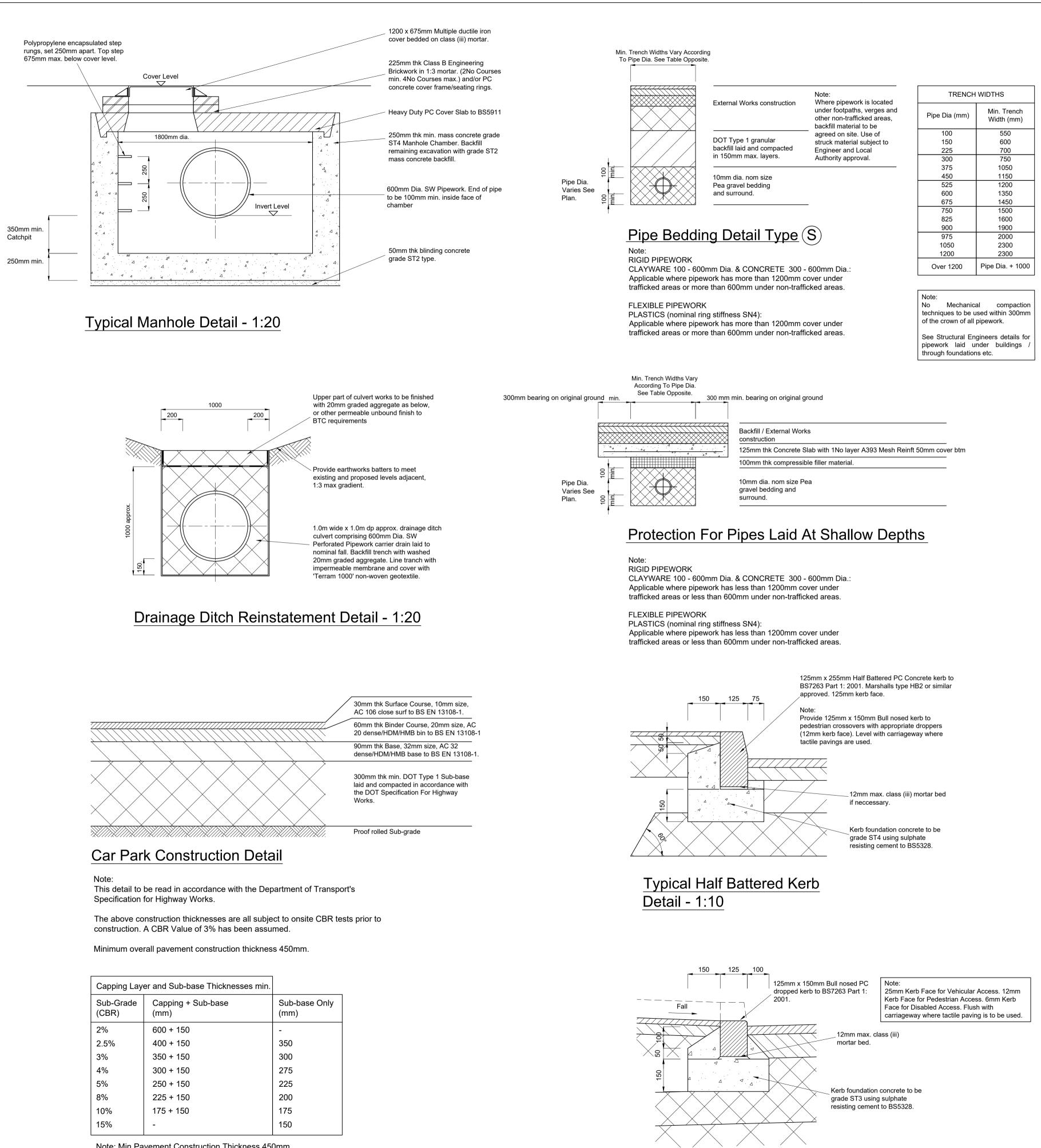
Note: Min.Pavement Construction Thickness 450mm
