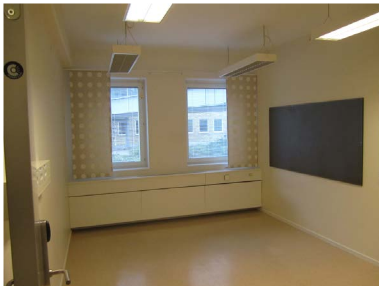
Picture 2: showing a view from the access door. All light fittings will be removed to ensure the required working height of 2.1m can be achieved within the cleanroom.
