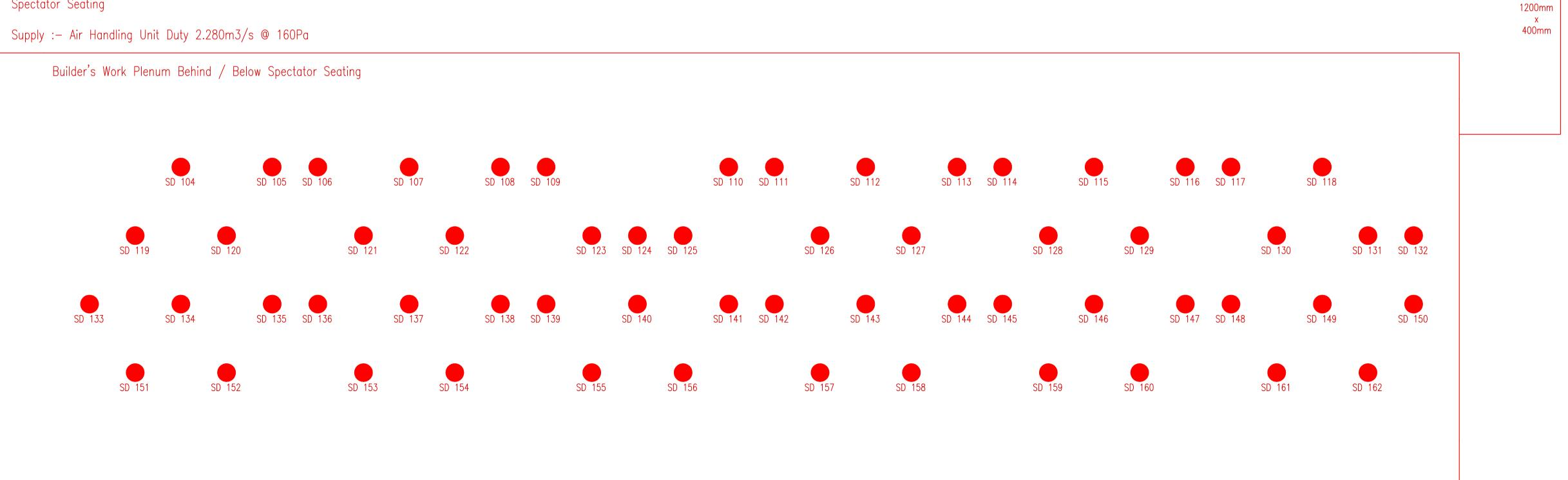
59 No. Supply Air Valves SD 104 to SD 162 inclusive fitted through concrete tier risers behind selected seats. Total Supply Air Volume Flow Rate 59 No. @ 0.035m3/s = 2.065m3/s
