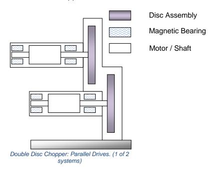
The full Specification provides the requirement for a total of four chopper discs to be purchased following placement of the contract.
