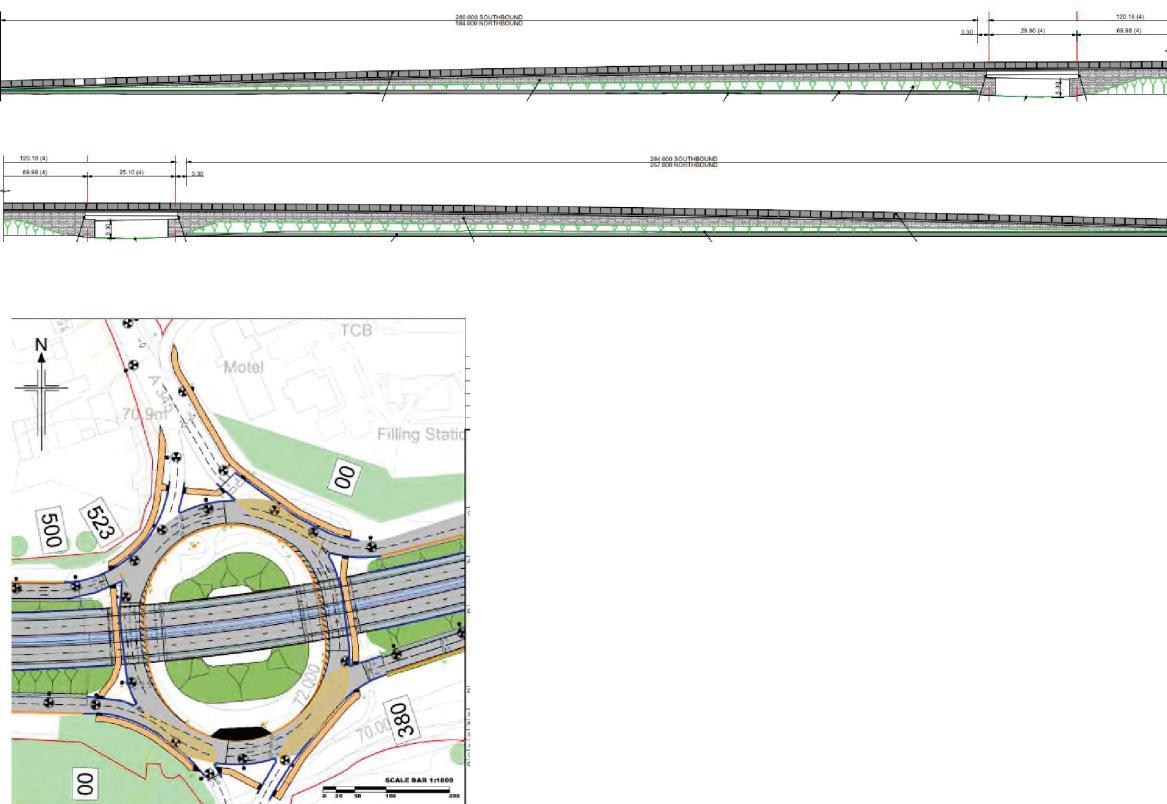
Bridge abutments are being designed to support the bridge superstructure on a spread foundation (bankseat) constructed directly on top of the reinforced soil zone. The selected solution will depend on the bearing capacity of the foundation soil and the probable need for ground improvement.
