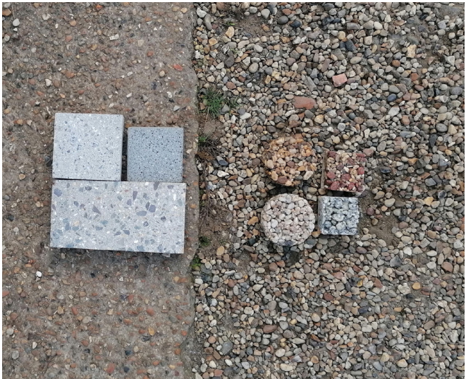
Testing samples of gravel options and step materials on site against existing loose gravel and concrete with exposed aggregate
