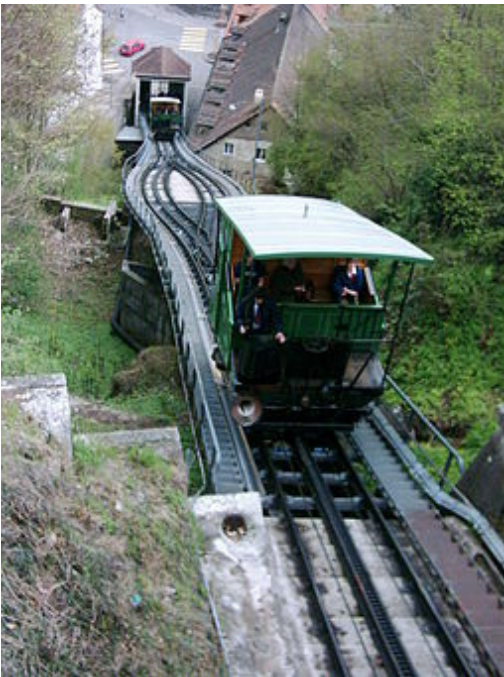
Image 3- A Funicular using waste water in Fribourg, Switzerland
