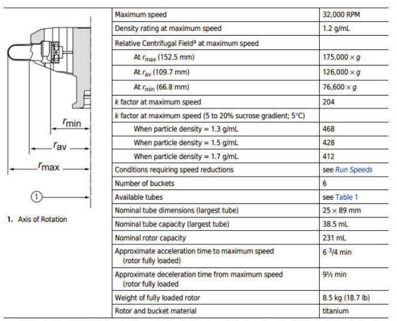
a. Relative Centrifugal Field (RCF) is the ratio of the centrifugal acceleration at a specified radius and speed ( $r\omega^2$ ) to the standard acceleration of gravity (g) according to the following formula: RCF =  $r\omega^2/g$  — where r is the radius in millimeters,  $\omega$  is the angular velocity in radians per second (2  $\pi$  RPM /60), and g is the standard acceleration of gravity (9807 mm/s<sup>2</sup>). After substitution: RCF = 1.12r (RPM/1000)<sup>2</sup>
