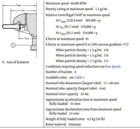
a. Relative Centrifugal Field (RCF) is the ratio of the centrifugal acceleration at a specified radius and speed ( $r\omega^2$ ) to the standard acceleration of gravity (g) according to the following formula: RCF =  $r\omega^2/g$  — where r is the radius in millimeters,  $\omega$  is the angular velocity in radians per second (2  $\pi$  RPM /60), and g is the standard acceleration of gravity (9807 mm/s<sup>2</sup>). After substitution: RCF = 1.12r (RPM/1000)<sup>2</sup>
