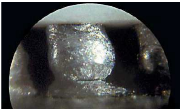
Figure 16-19: BGA – Unacceptable, fractured solder joint
