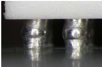
Figure C-1: Typical CBGA solder joint (high melting point balls)
