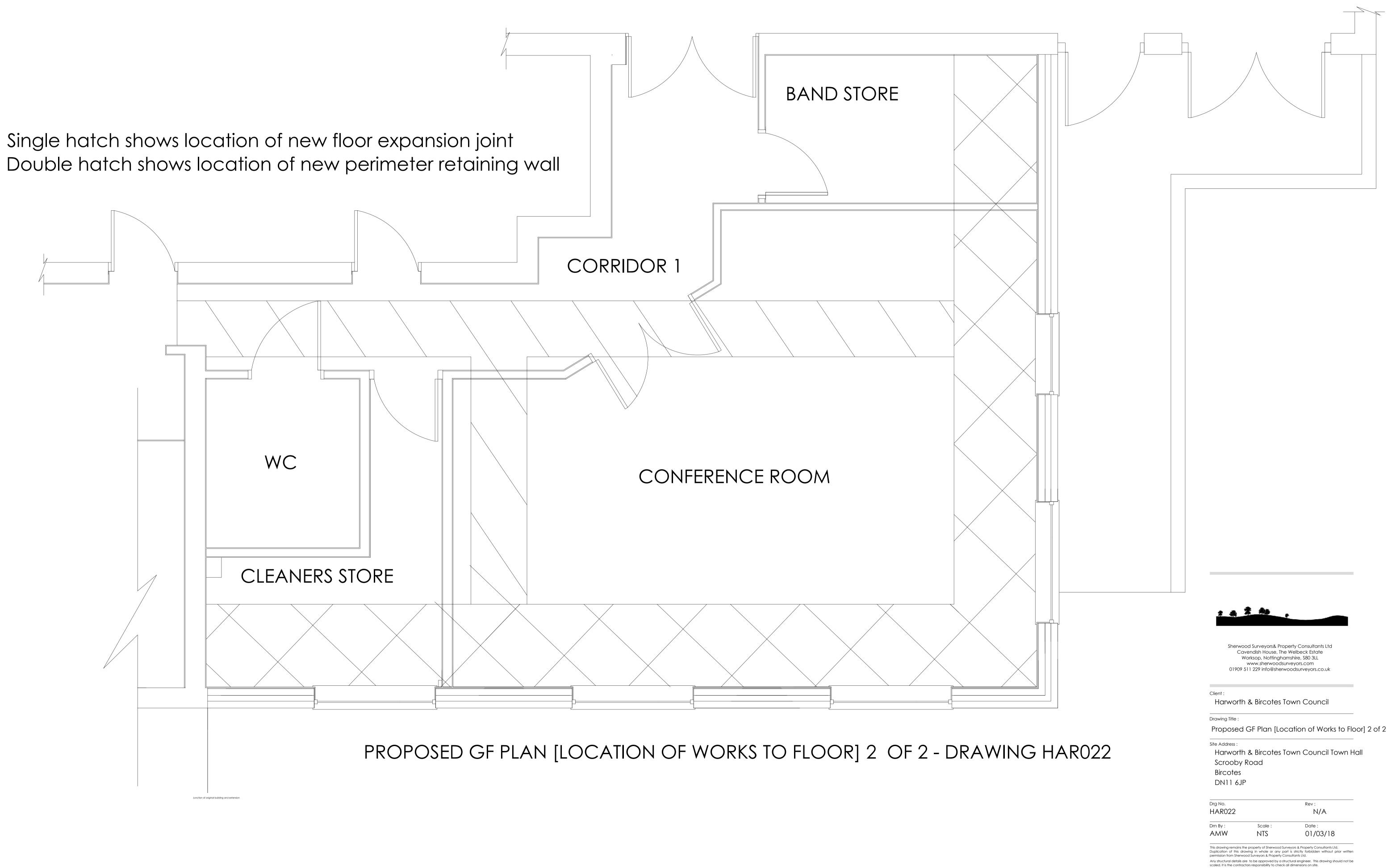
Single hatch shows location of new floor expansion joint
