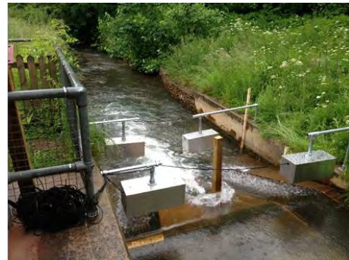
Images of recessed eel tiles at Burnt Mill gauging weir and testing of mounted and recessed tiles at Lydney.
