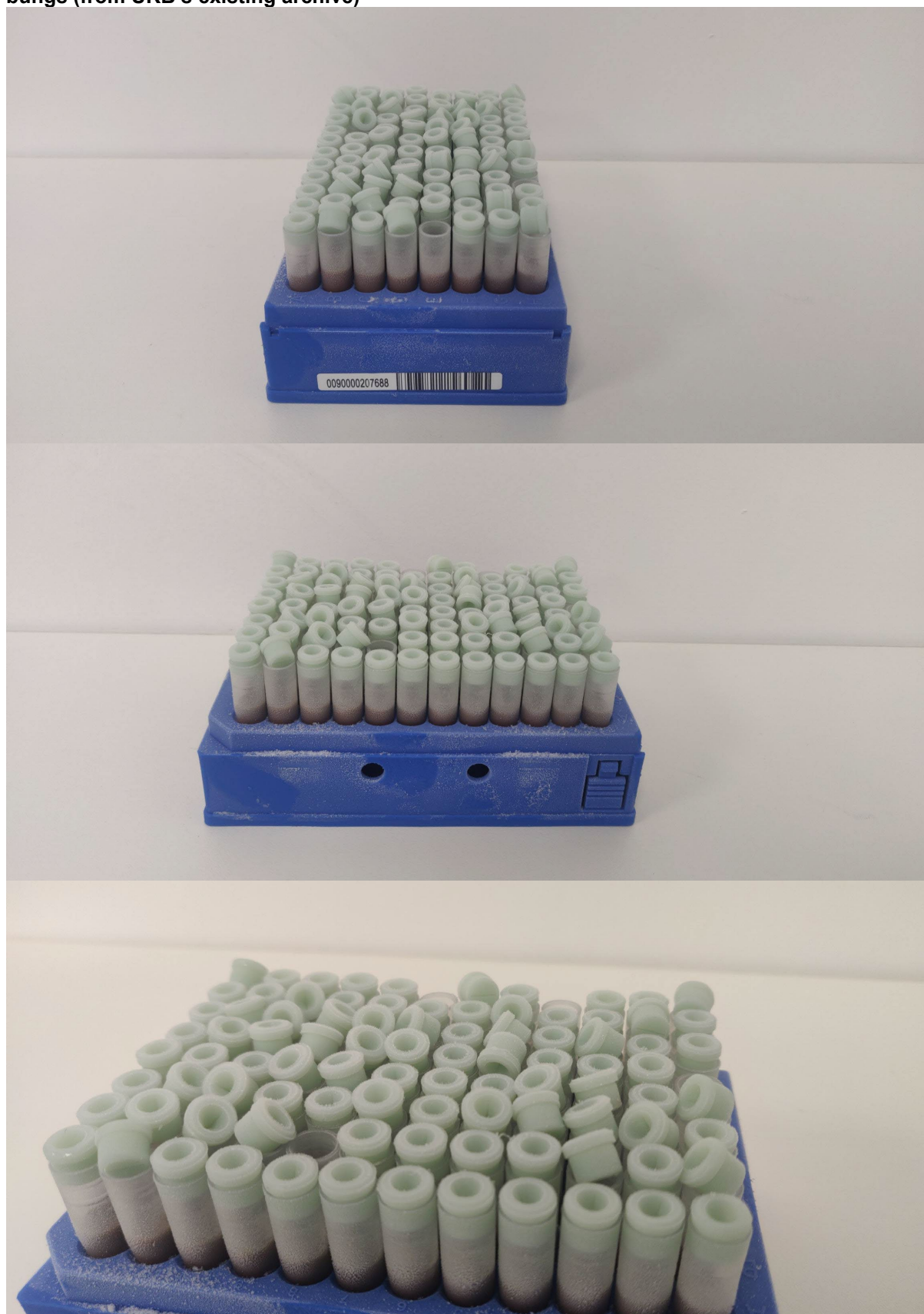
Example of an ABGene Rack with a particularly high density of raised and loose septum seal bungs (from UKB's existing archive)
