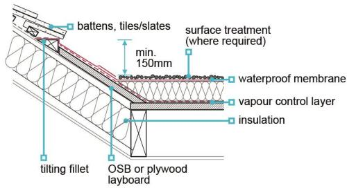
**Please note** - Strip back roof to form pitched-flat abutment; apply 12mm sarking boards, 25mm stop batten, dress single ply up and over stop batten, fit on fascia eaves ventilator equivalent to 10,000mm2 /lm (if roof ventilated) dress breather membrane over and lodge bottom plain tile. Note, eaves insulation tray ventilator may be required to maintain airflow.
