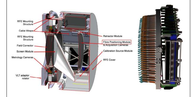
This tender is for the design, manufacture and assembly of the FPU mechanism only. The scope of the procurement does not include provision of electronics or the optical fibre.
