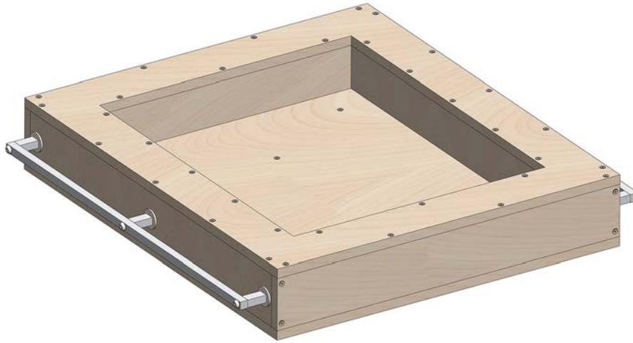
**Figure 25: Stab backing material container**
