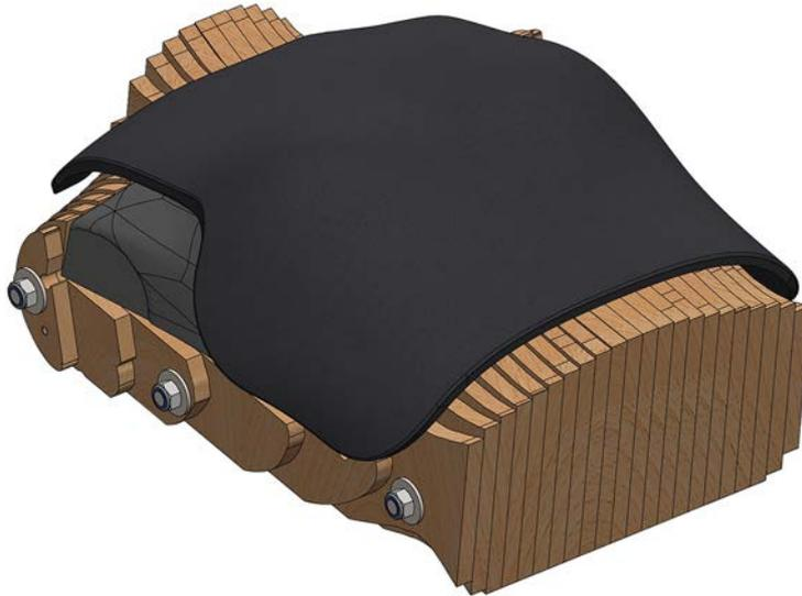
**Figure 31: Formed armour stab test configuration**
