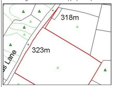
Polygons must not contain "bowties". Polygons must not intersect or cross themselves. In the figure below the digitised field has a bowtie caused by a polygon crossing itself:
