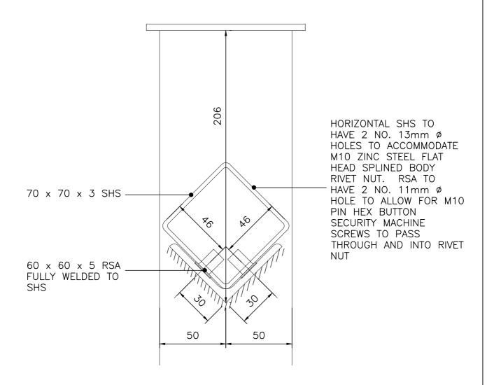
SIDE VIEW - HORIZONTAL RAIL SECURING DETAIL - 1:2
